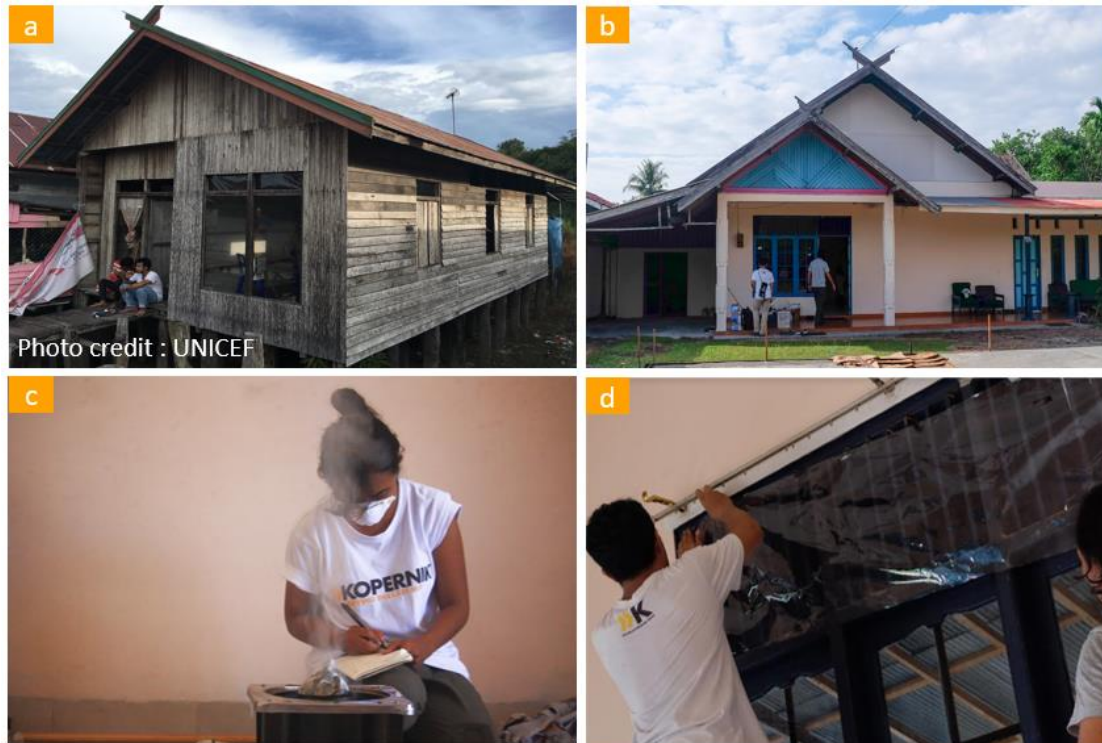
Figure 4. Field tests carried out in two types of houses. a) First test site in a wooden house in Petuk Katimpun village. b) Second test site in a beton house in Palangka Raya city. c) Smoke generated from burning fuel in a cookstove. d) Sealing ventilation spaces in a beton house.
