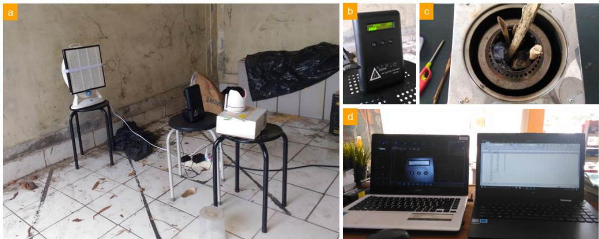
Figure 3. Preliminary test setup. a) Devices arranged in the garage. b) Dylos particle counter to measure PM_{2.5} level. c) Cookstove with paper, wood and tissue as fuel for smoke source. d) Continuous remote monitoring during the tests
